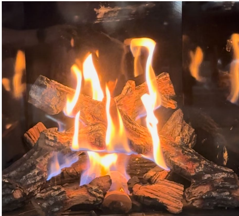
Figure 6-2 Burner Flame Heights: This image provides a visual reference for the burner flames burning at maximum height after the burners have been operating for 30 minutes or longer. This, however, is dependent on the gas type, air shutter opening setting and vent system configuration. Actual flame heights can be slightly higher or lower when compared to this reference image.
